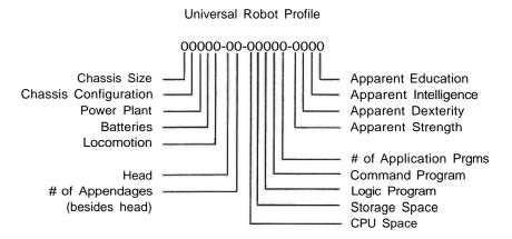
The codes used for the URP digit positions describing chassis size, chassis configuration, power plant, batteries, locomotion, logic program, and command program come directly from the design tables.
